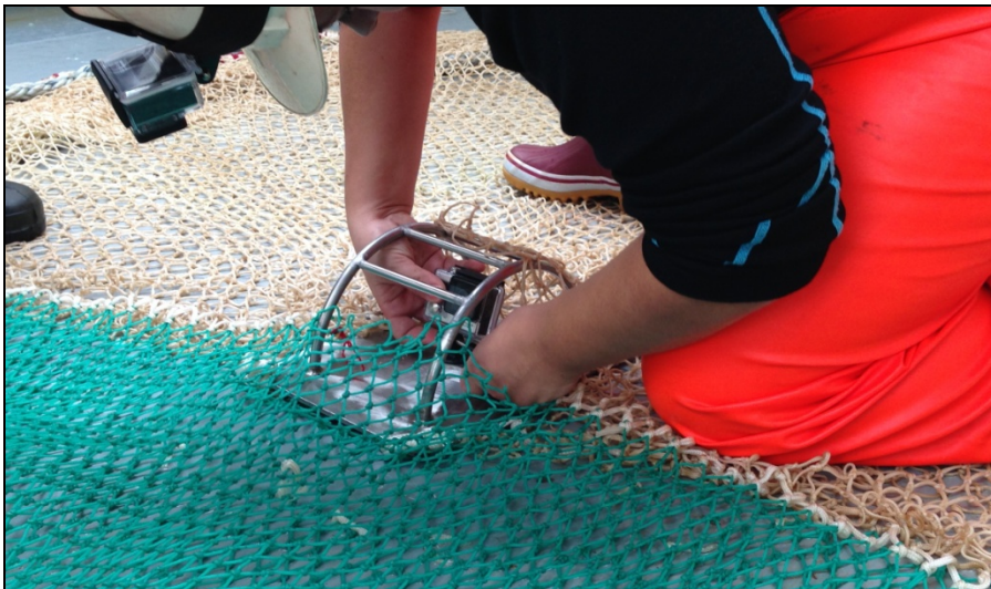
Photo 2. GoPro camera attached to inside of trawl by fish lock on Finnur Fríði. The steel frame was tied to trawl, at the each corner using a rope.
